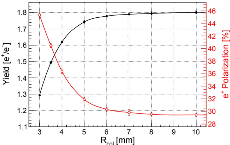
$$P_{e^+ \text{ max}} \simeq 40\% \text{ for } R_{\text{col}} = 3.5 \text{ mm}$$
