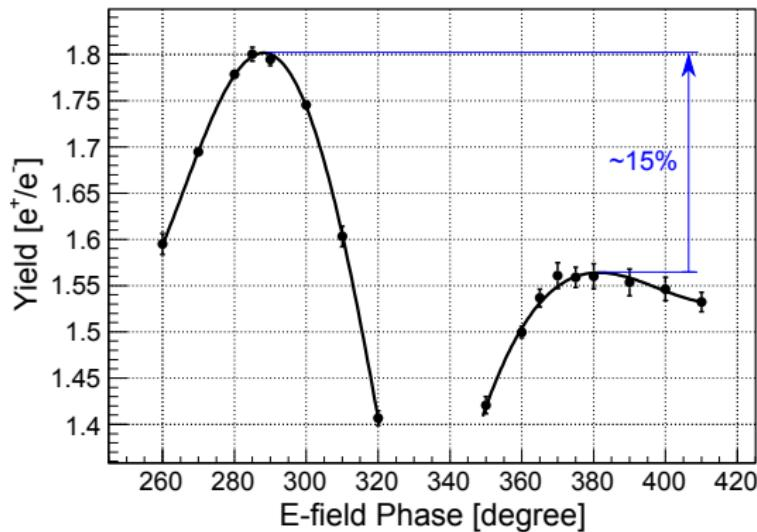
Proper choice of capture RF phase (only!) allows to use e<sup>+</sup> source down to **120 GeV e<sup>-</sup>** (*without any additional modifications*)
