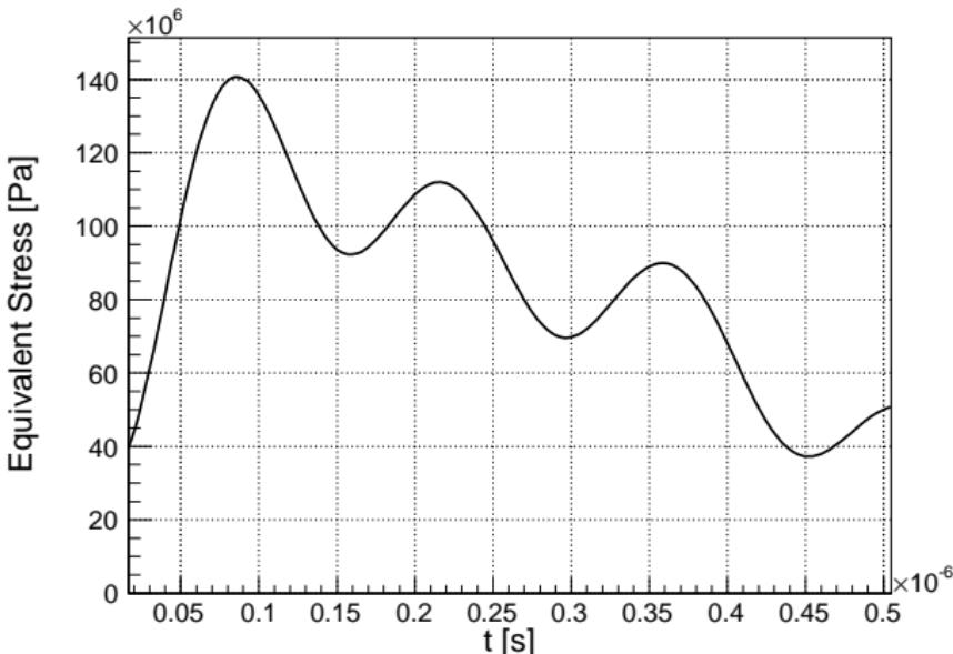
Max. Equivalent Stress:  $\simeq 140$  MPa (27.5% of Fatigue Strength)
