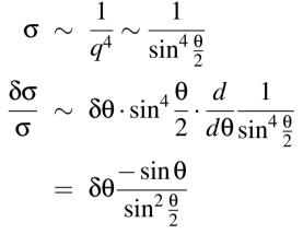
$\Rightarrow$  to measure cross sections to 1% at  $\emph{e.g.}$   $\theta=20^{\circ}$  we need an angular resolution of
