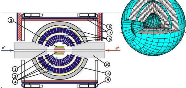
1 – beam pipe, 2 – tracking system, 3 – aerogel Cherenkov counter, 4 – NaI(Tl) crystals, 5 – phototriodes, 6 – iron absorber, 7-9 – muon detector, 10 – focusing solenoids.
