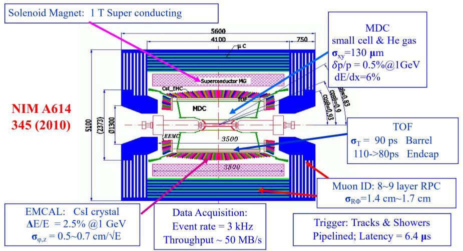
Hermetic spectrometer for neutral and charged particle with excellent resolution, PID, and large coverage
