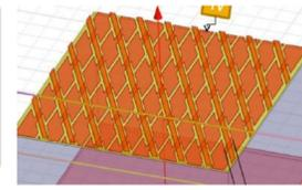
Anode plane with jagged strips to reduce of around 30% inter-strip capacitance (MAXWELL simulations)
