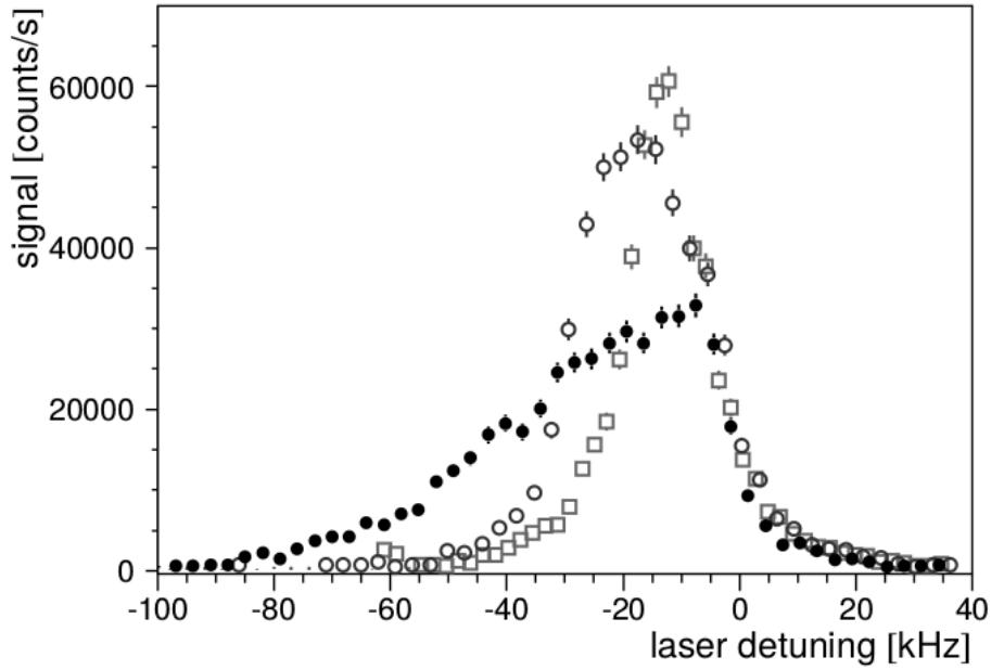
FIG. 4. Doppler-free spectrum of normal fraction above and below the onset of BEC. The symmetric spectrum (above  $T_c$ , open symbols) suddenly becomes asymmetric (solid symbols) when the condensate forms. Temperatures for the three spectra are about 120  $\mu$ K (open squares), 53  $\mu$ K (open circles), and 44  $\mu$ K (solid circles).
