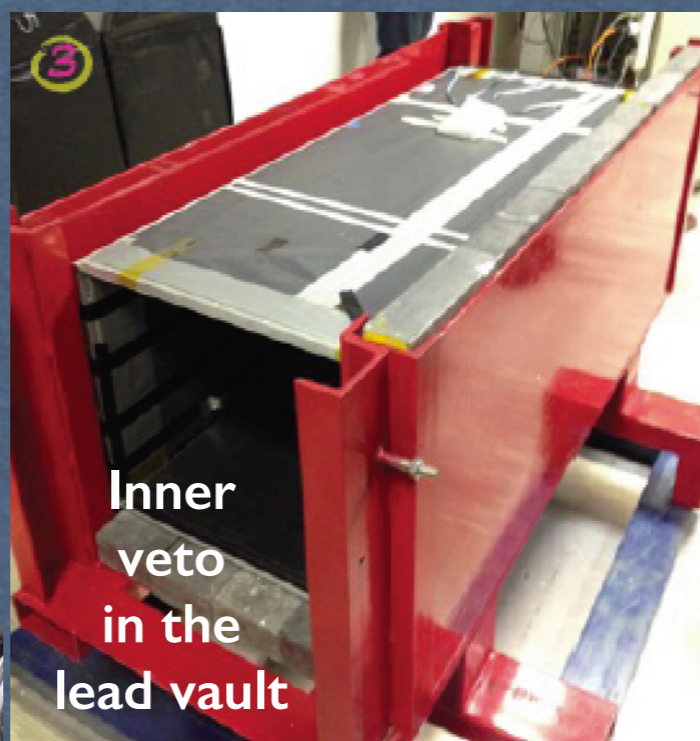
Inner veto plastic scintillators paddle + WLS + SiPM
