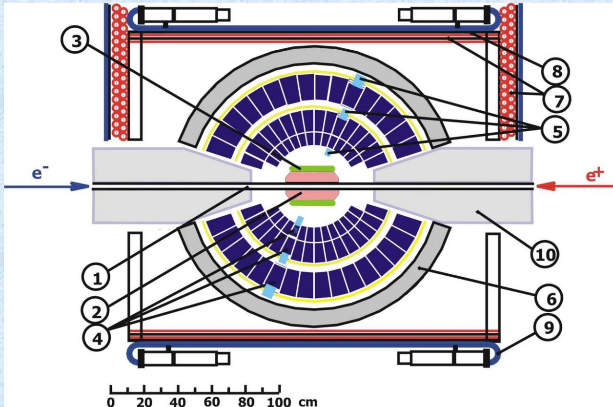
1 – beam pipe, 2 – tracking system, 3 – aerogel counters, 4 – NaI(Tl) crystals, 5 – phototriodes, 6 – iron muon absorber, 7–9 – muon detector, 10 – focusing solenoids.
