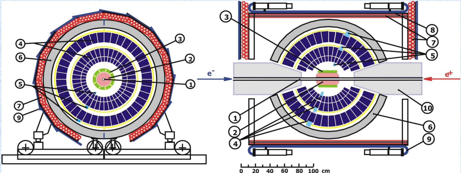
1 – beam pipe, 2 – tracking system, 3 – aerogel Cherenkov counters, 4 – NaI(Tl) crystals, 5 – phototriodes, 6 – iron muon absorber, 7–9 – muon detector, 10 – focusing solenoids.
