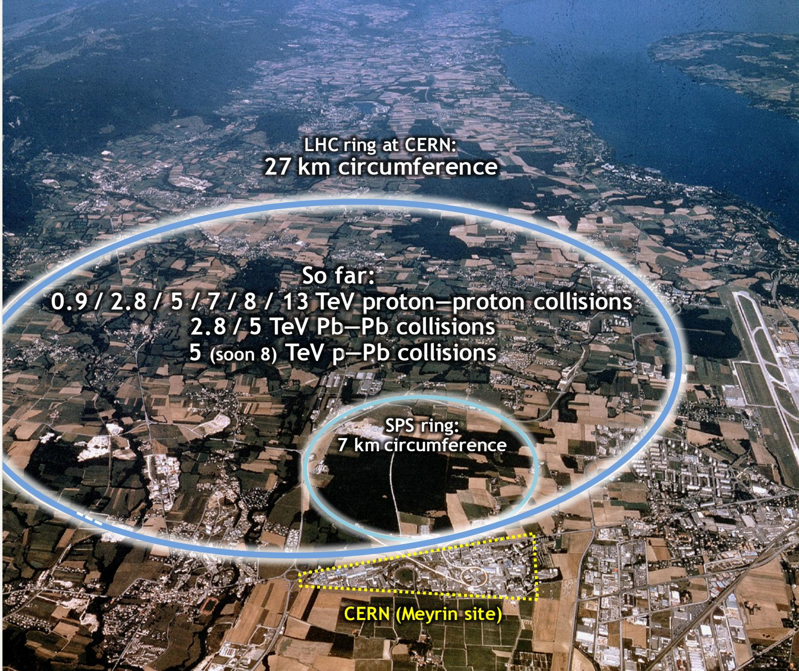
~20 minutes are required to accelerate the protons in the LHC from 450 GeV to 7 TeV
