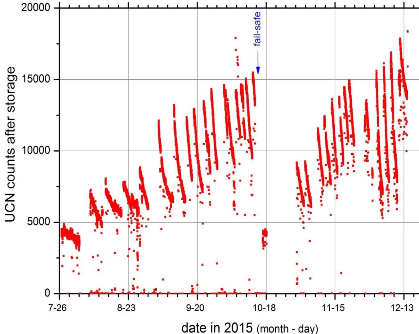
Measurement of the total UCN counts (spin-up and -down) after 180s of storage in the nEDM precession chamber
