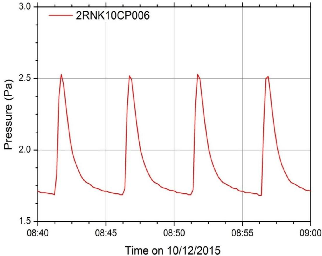
D2 vapor pressure shows cooling works also fine at higher duty cycle
