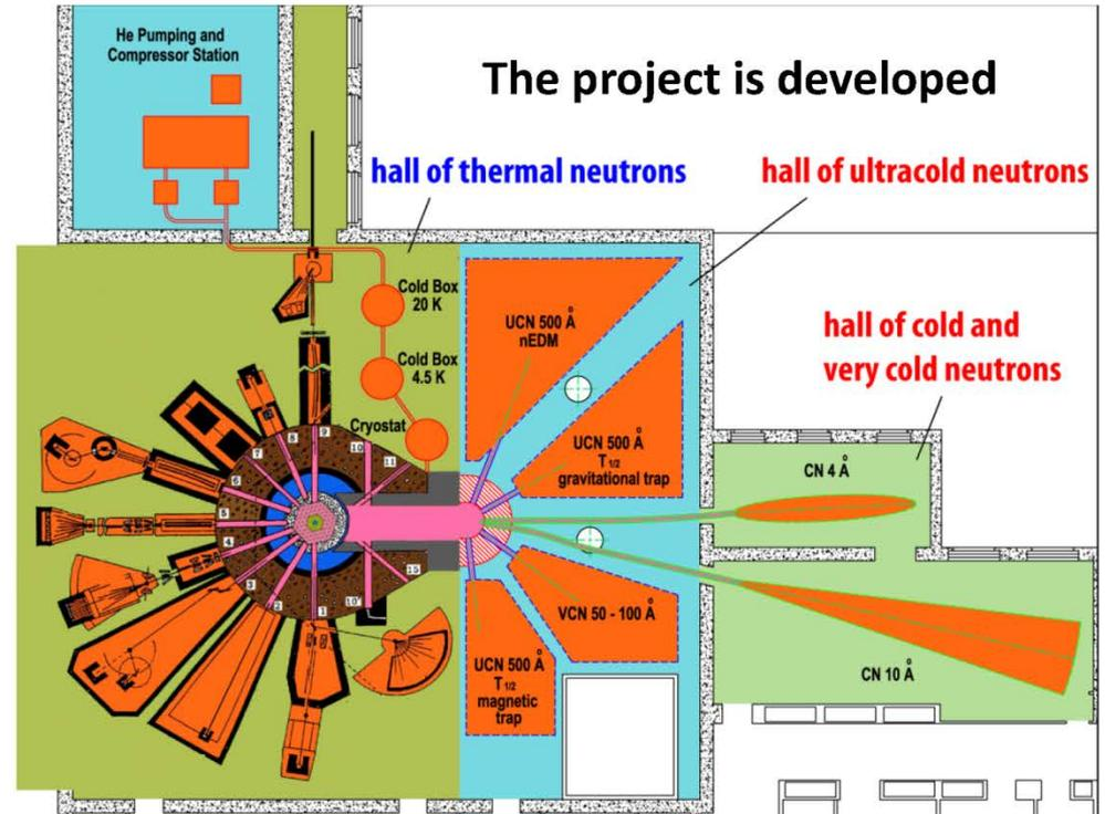
The scheme of experimental installations on the WWR-M reactor after installation in a thermal column of the reactor of UCN source with superfluid helium at a temperature of 1.2K.
