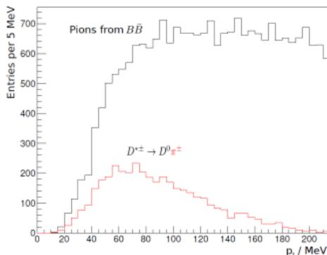
Figure : Transverse momentum distribution of pions from  $D^{*\pm}$  and  $B\bar{B}$  decays
