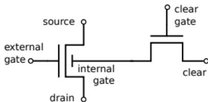
Figure : Equivalent circuit of the DEPFET pixel
