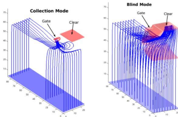
Figure : Simulation of electron trajectories in the detector
