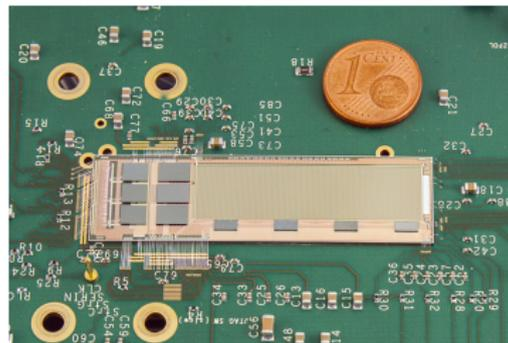
Figure : Hybrid6 module: 480x192 px (2013)
