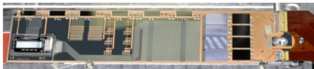
Figure : Electrical Multi Chip Module: electrical prototype (2013)
