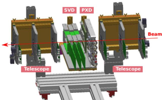
Figure : Beam test setup with a VXD segment, DESY 2014
