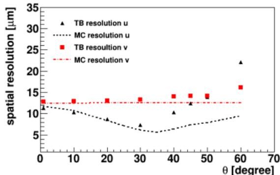
Figure : Resolution of the DEPFET sensor
