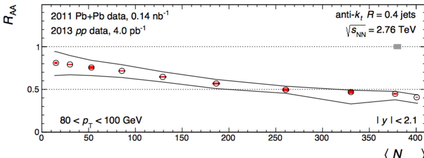
$R_{\text{AA}}$ : jet nucleon modification factor; ratio of yields (heavy ion / pp)
