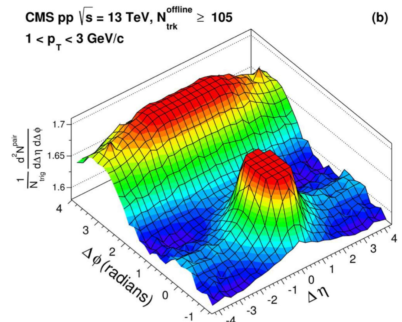
two-particle correlations, confirming the presence of a ridge-like structure for same-side ( $\Delta\phi \sim 0$ ) pairs in high-multiplicity events at 13 TeV. (arXiv:1510.03068)
