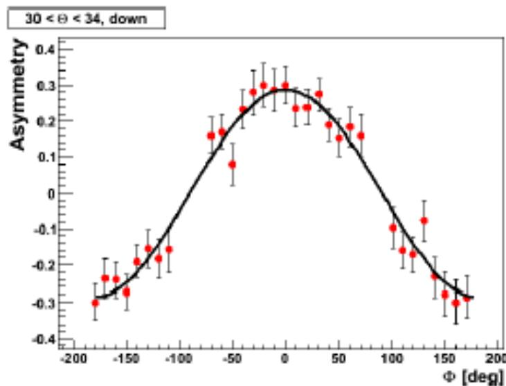
$$\frac{N(\theta, \varphi) - N(\theta, \varphi + \pi)}{N(\theta, \varphi) + N(\theta, \varphi + \pi)} \equiv \epsilon(N(\theta, \varphi), N(\theta, \varphi + \pi))$$
