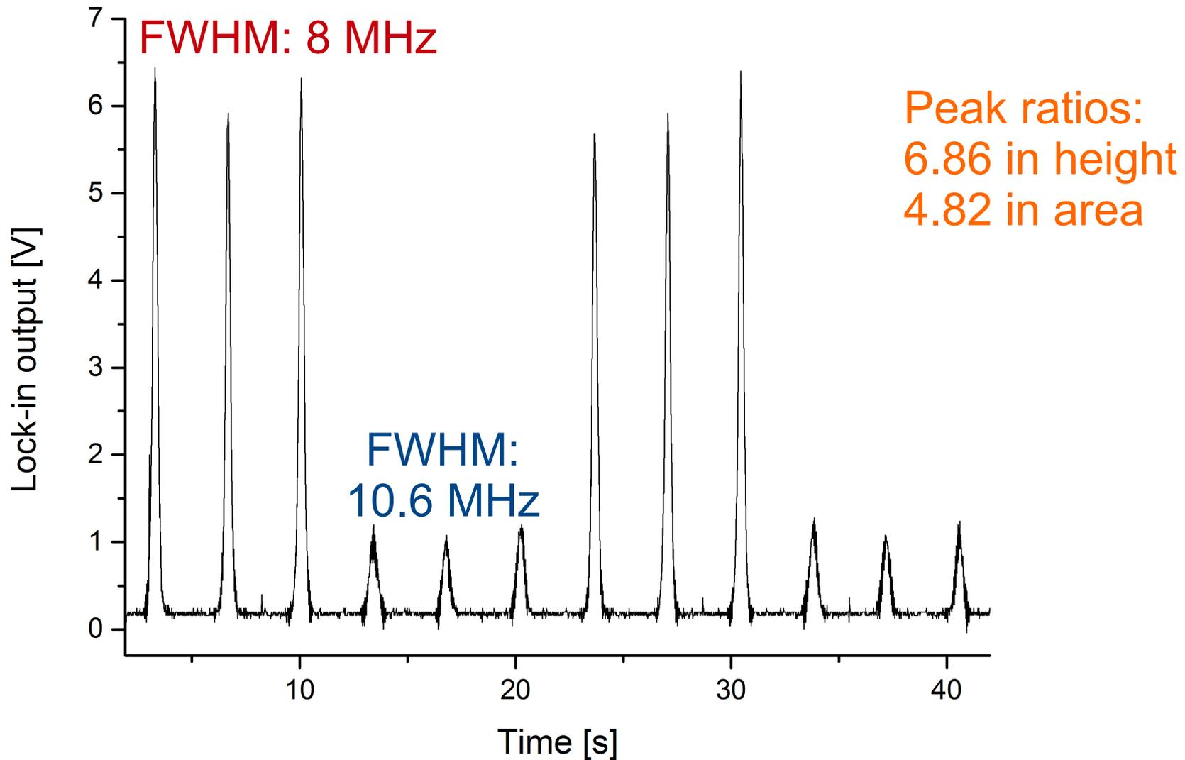
Scan 408 laser 100 MHz in 3.4 s, lock-in time constant 3 ms
