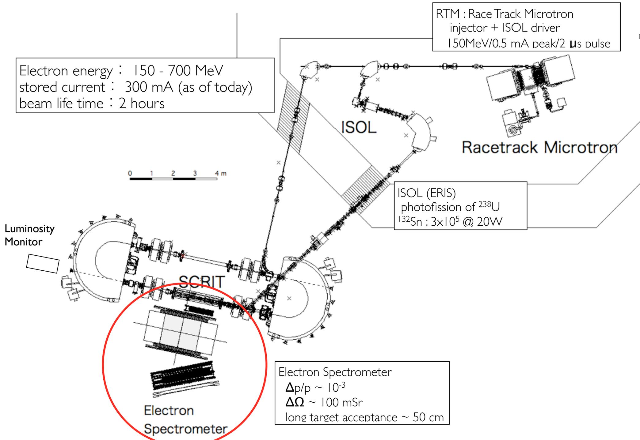
(Window-frame Spectrometer for Electron Scattering)
