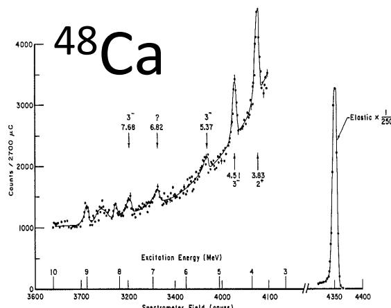
Fig. 7. Spectrum of electrons scattered from  $\text{Ca}^{48}$ . The incident energy is 60.1 MeV and  $\theta=130^\circ$ . The spectrum has been corrected for background.
