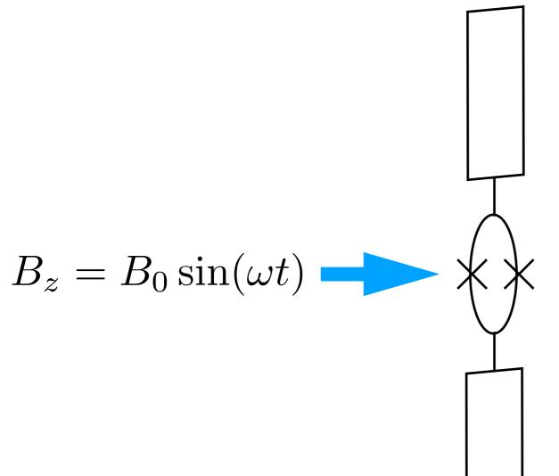
Flux modulates qubit level spacing:
