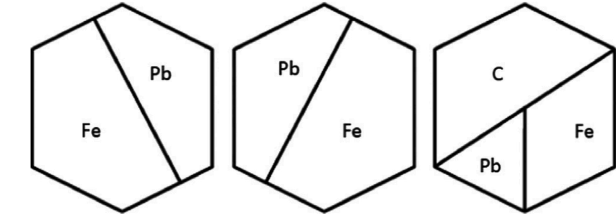
**Fig. 3.** Orientation of the nuclear targets looking downstream. Targets 1 and 5 have the leftmost orientation, target 2 has the middle orientation, and target 3 the rightmost orientation.
