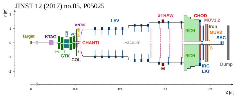
400 GeV/c protons from the SPS on a beryllium target produce secondary charged beam: 6% are 75 GeV/c K<sup>+</sup> mixed with  $\pi^+$  (70%) and protons (23%), 1% momentum spread (rms), ~100 µrad divergence.
