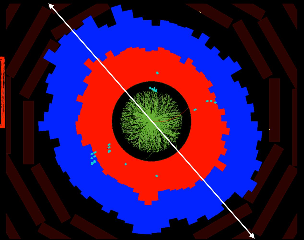
Transverse energy flow in CMS calorimeters for single Pb+Pb collision at 2.76TeV
