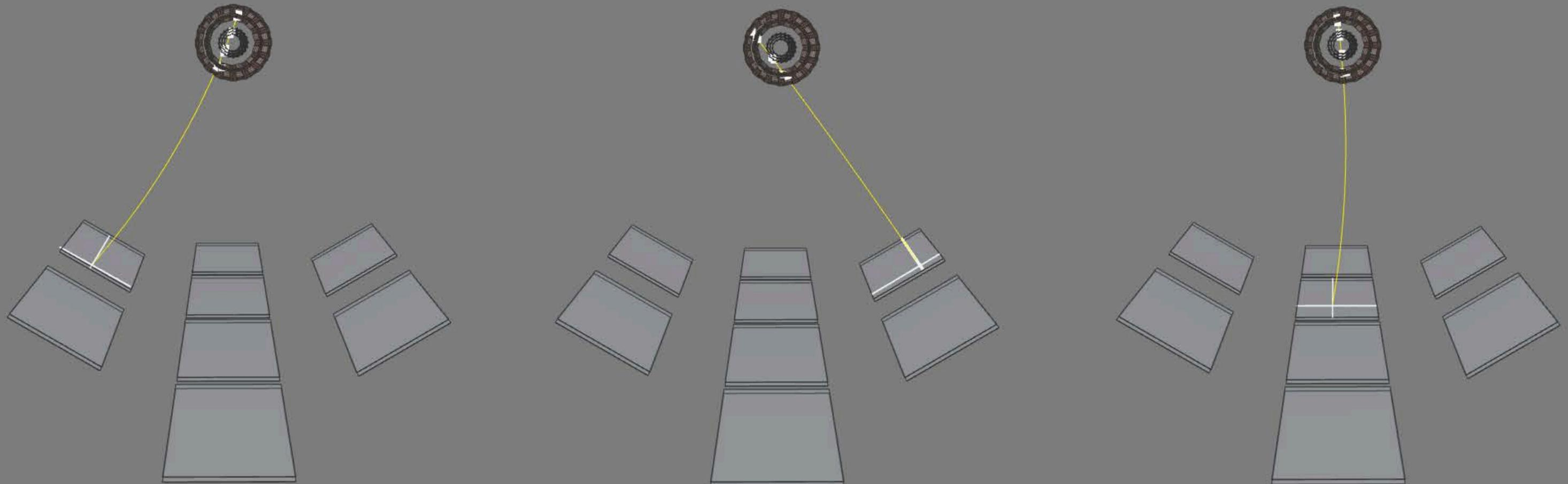
Matching of cosmic ray muon tracks from inner silicon detectors to microMega TPC outer tracker → essential tool for correction of TPC space charge distortions
