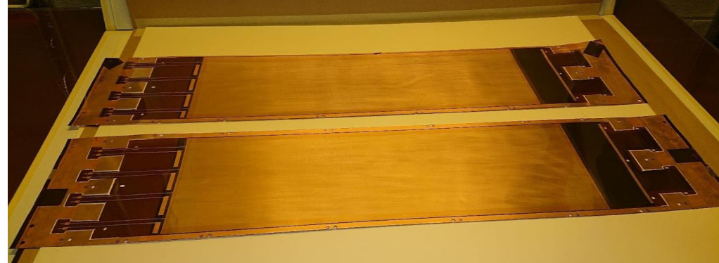
Flexible Micro-RWELL PCB produced at CERN-EP-DT MPT Workshop. Each foil is divided in four HV sectors
