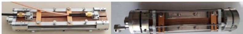
Figure 4.5: Photographs of the cavity halves installed in tuning holding structure with gears. Top view (left) and bottom view (right).
