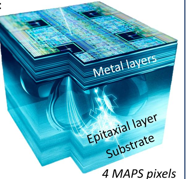
**Stitching** will be used: repeated identical but functionally independent units, with **in-silicon interconnections** and peripheral structures along the outer edges of the resulting large-area chip.
