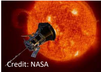
Credit: NASA Size of PSP ~ 1.0 × 3.0 × 2.3 m (685 kg → 555 kg)
