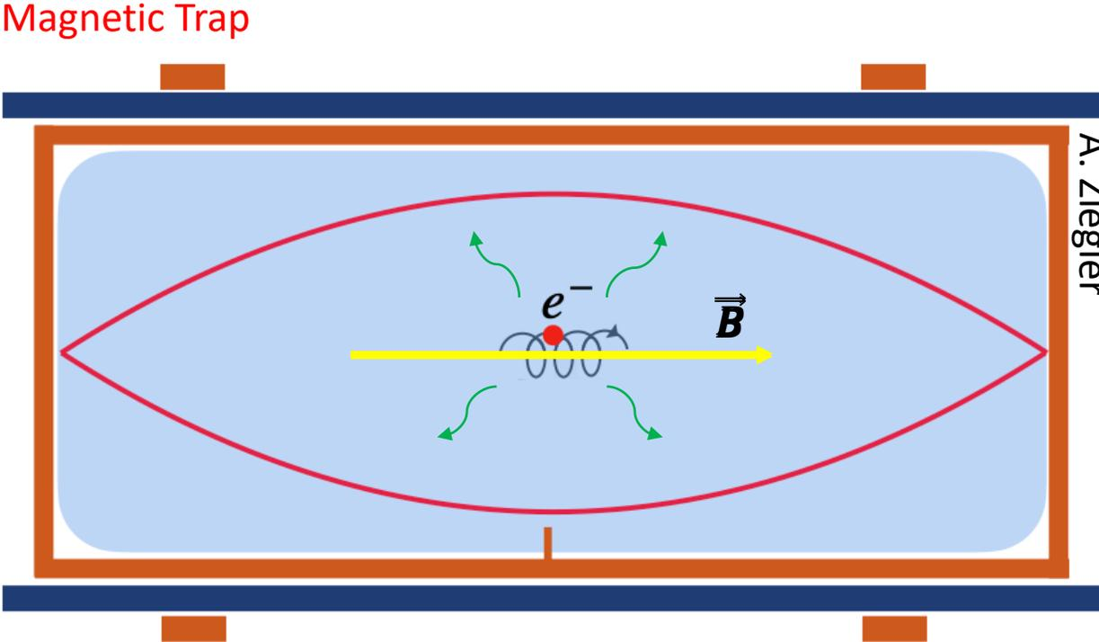
Radiation detected with resonant cavities
