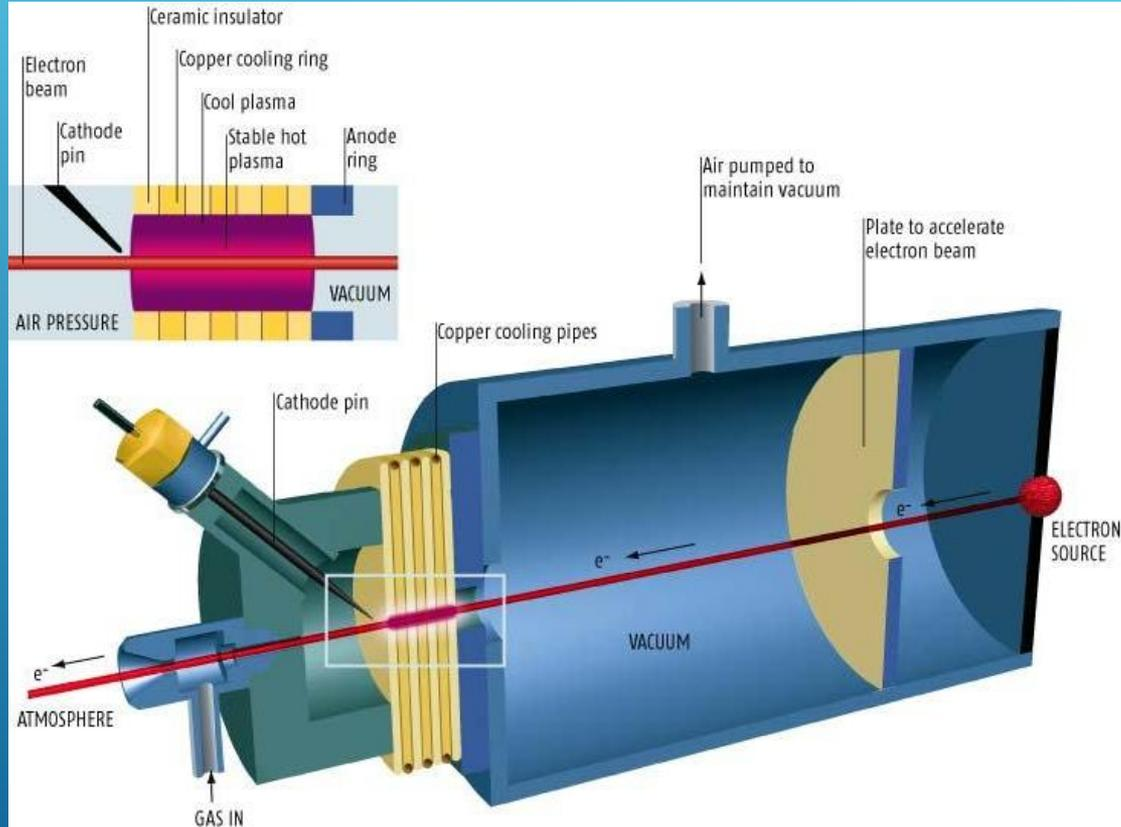
The stabilized plug of plasma seals the vacuum chamber to air but allows particle beams to pass through
