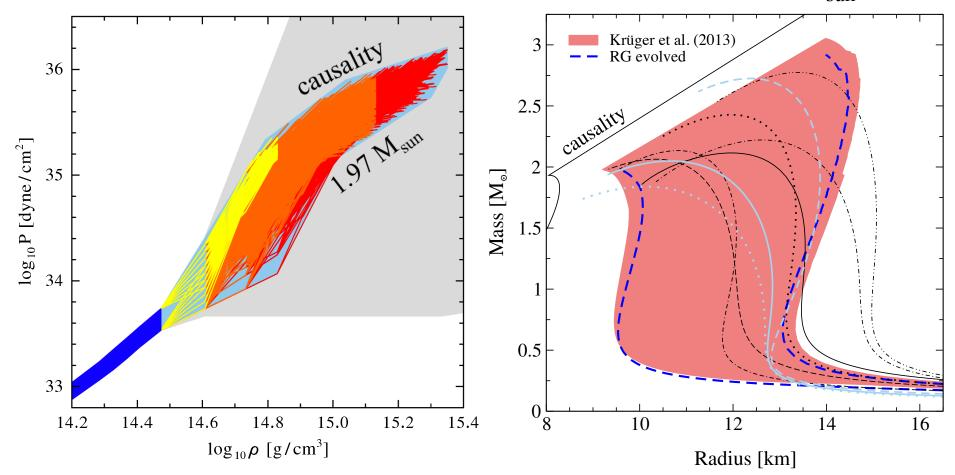
low-density pressure sets scale, chiral EFT interactions provide strong constraints, ruling out many model equations of state
