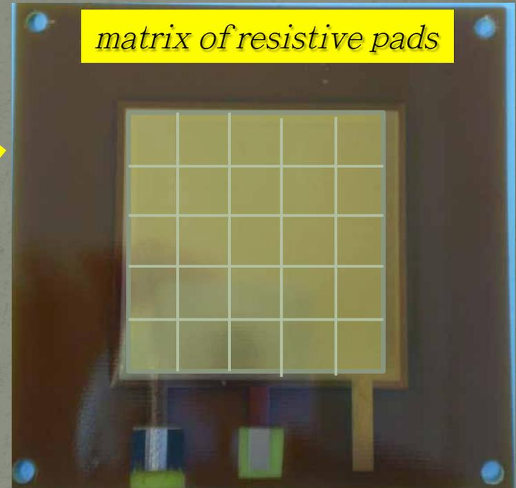
The rate capability of the detector, for a fixed surface resistivity, can be tuned with a suitable segmentation (NIMA 732(2103)199) of the resistive layer (under study): a “matrix of resistive pads” each one independently connected to ground ( $\sim 1 \text{ MHz/cm}^2$  for m.i.p. seems achievable)
