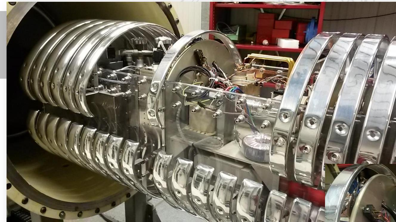
**Beam Energy:** 40-400 kV (absolute value  $\pm 0.3 \text{ keV}$ , spread  $< 0.1 \text{ keV}$ )
