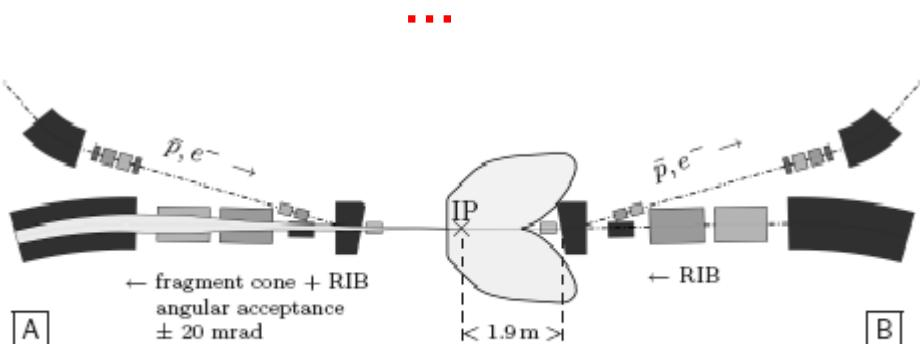
Figure 6: Interaction zone with the interaction point IP in the bypass section of the NESR.
