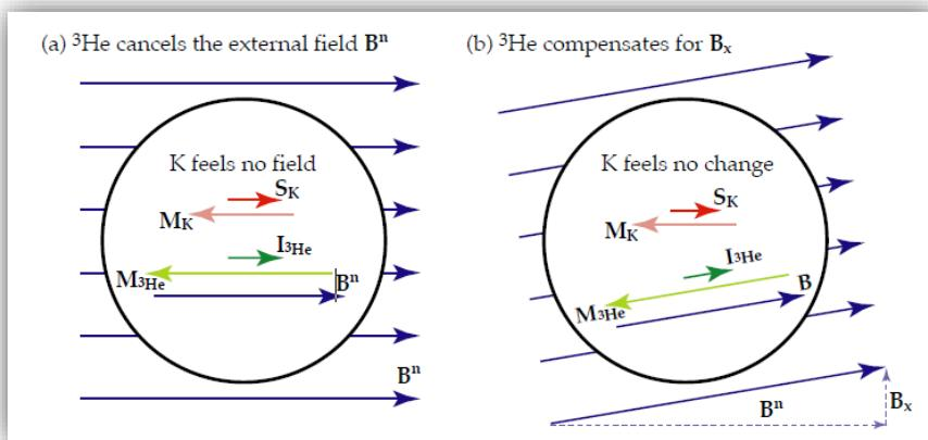
Romalis's self-compensating magnetometer
