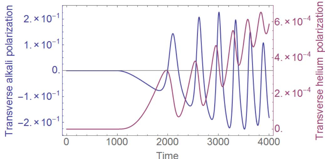
**Transverse magnetic field causes rotation of both polarization**
