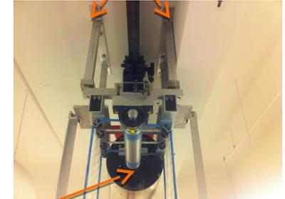
A Yaskawa 4kW servo motor smoothly raise/lower the two 210 kg Pb weights through a distance of 0.5m in 1s.
