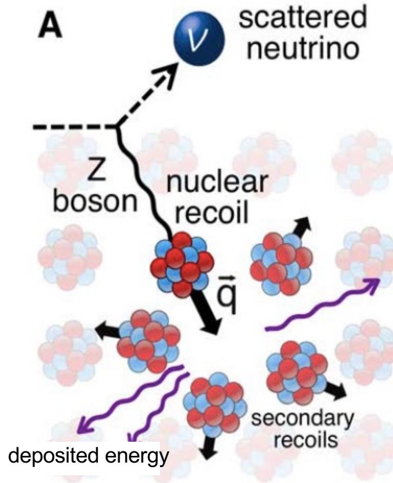
→ detectors developed over the last ~few decades are sensitive to ~ keV to 10's of keV recoils
