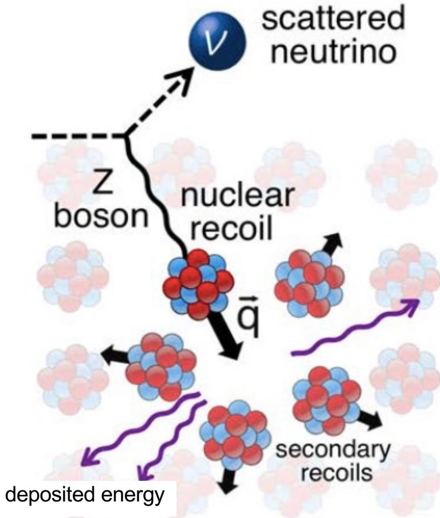
→ **WIMP dark matter detectors** developed over the last ~decade are sensitive to  $\sim$  keV to 10's of keV recoils
