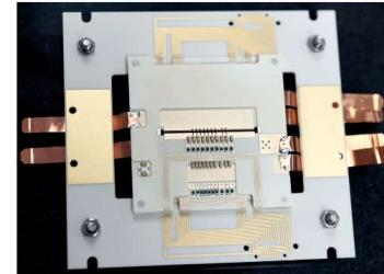
Trap for the group of **Prof. Andreas Schell (LUH)**. The trap will be used for levitation of nanoparticles to investigate if they behave in a classical way or in a quantum mechanical one.
