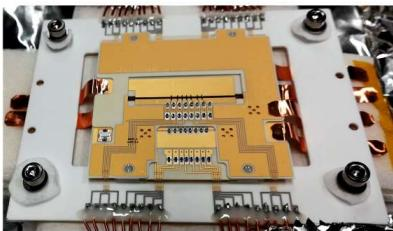
Trap for the group of **Prof. Kjeld Eikema (FU Amsterdam)**. The trap will be used for  $\text{He}^+$  1S-2S spectroscopy to test bound-state quantum electrodynamics and to search for new physics beyond the standard model.
