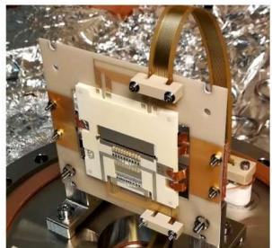
Trap for **Dr. Nils Huntemann (PTB)**. The trap is used for a  $\text{Yb}^+$  ion clock where the ions are sympathetically cooled with  $\text{Sr}^+$  ions.
