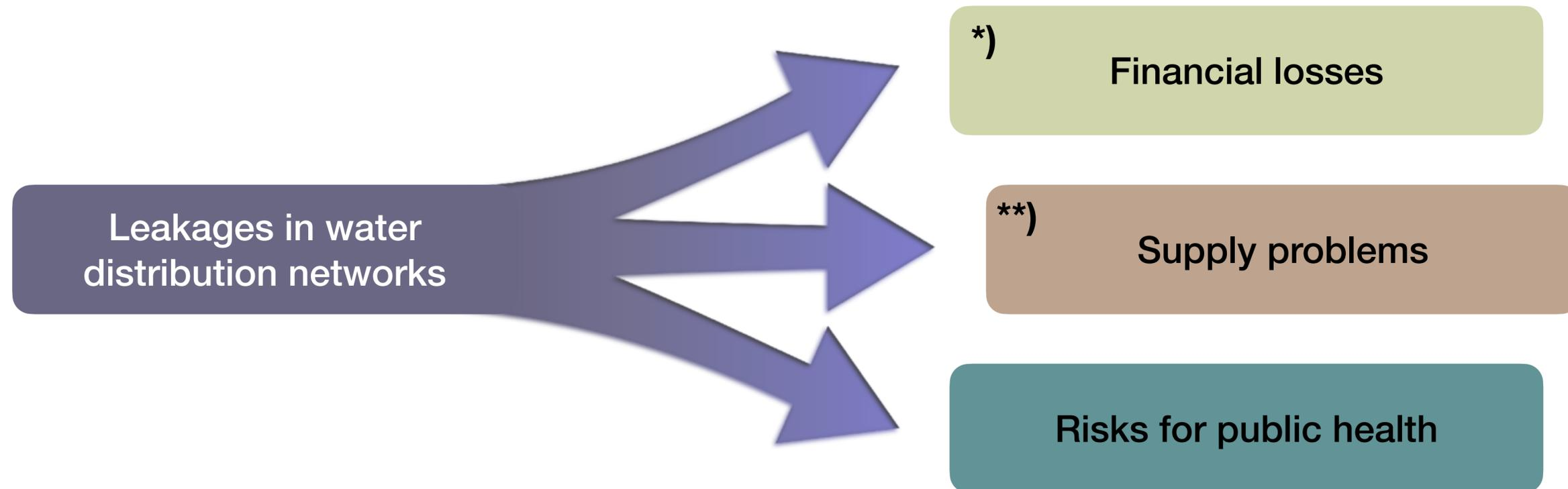
\* example: a 5 mm hole @ 5 bar leakages 32000 liters of water per day
