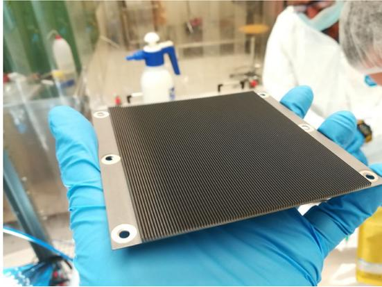
Grooved copper electrode sputtered with  $^{10}\text{B}_4\text{C}$  at the ESS Coating Workshop in Linköping (SE)
