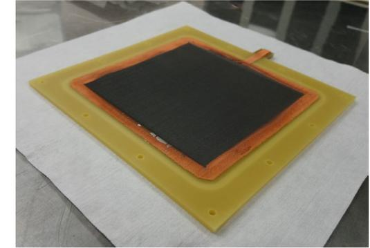
Metallic coated mesh to be inserted between cathode and amplification stage
