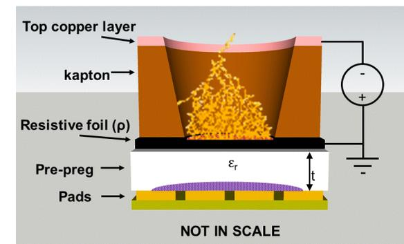
The "WELL" acts as a multiplication channel for the ionization produced in the gas of the drift gap
