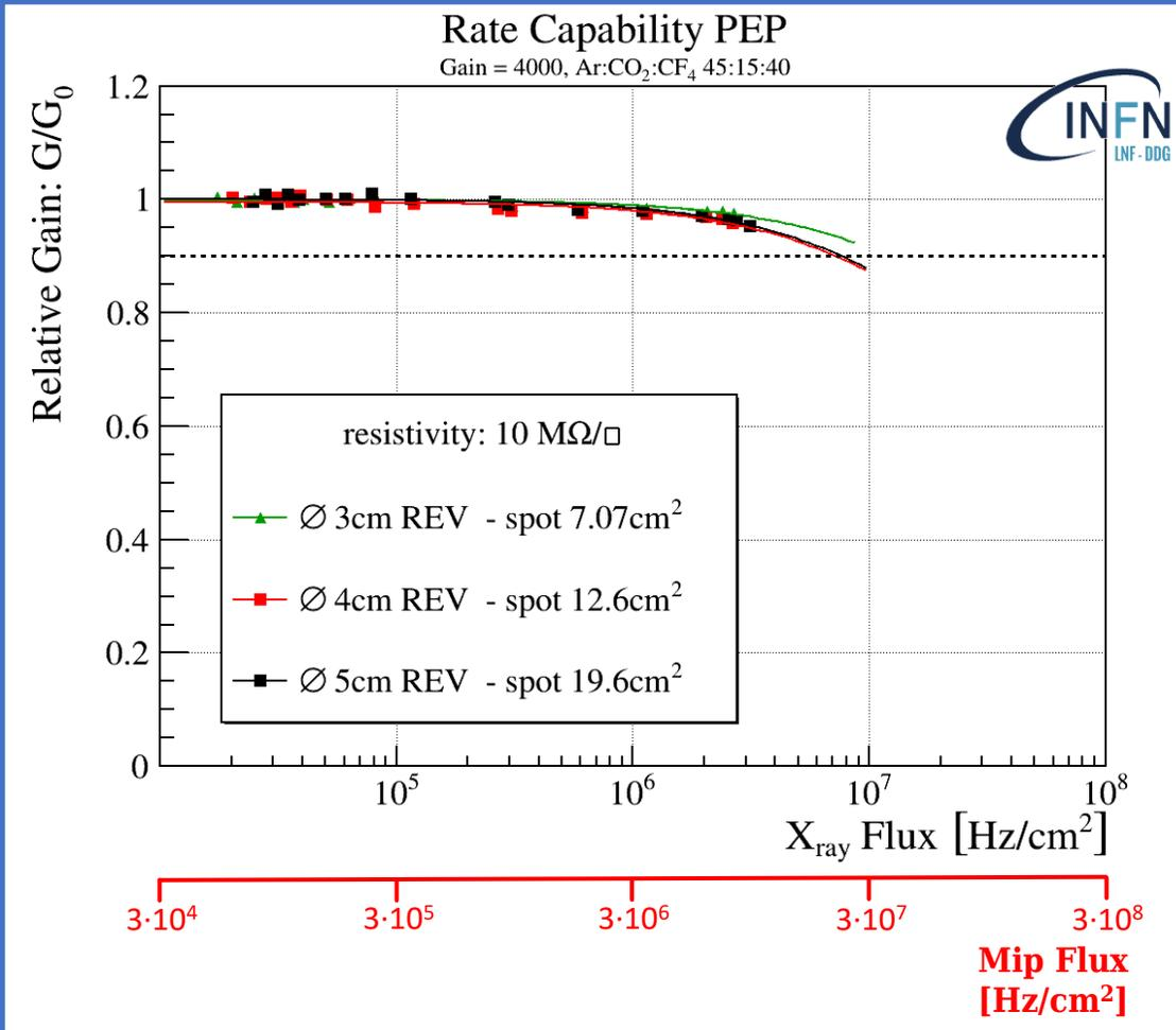
A rate capability under X-rays irradiation of 10 MHz/cm<sup>2</sup> (to be scaled by three for mip) is **extrapolated**.
