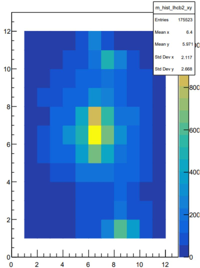
Beam profile reconstructed with the two chambers with PAD-segmented readout
