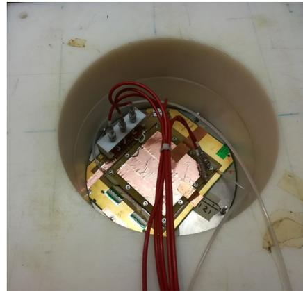
First data taking campaign: detector shaped to fit the small pit u-RWELL\_PCB re-drawn for the following tests.
