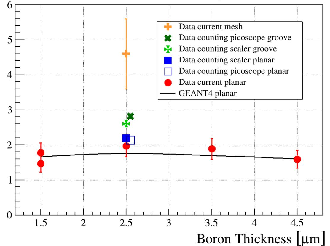
An efficiency up to 5% has been achieved for neutrons with average kinetic energy of 100 meV
