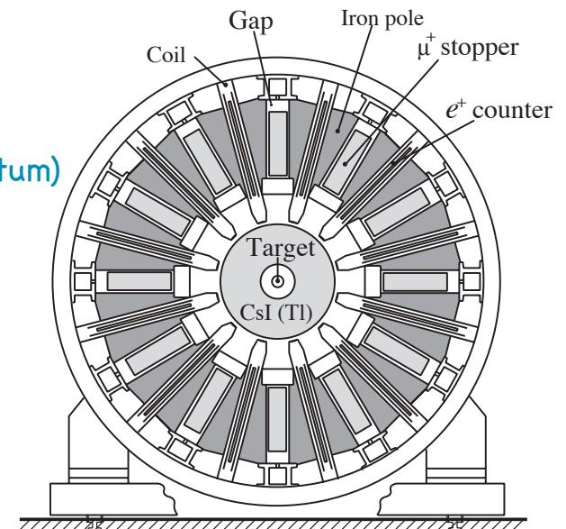
TREK detector: Upgrade of E246 detector for the study of various Kaon decay channels at J-PARC.
