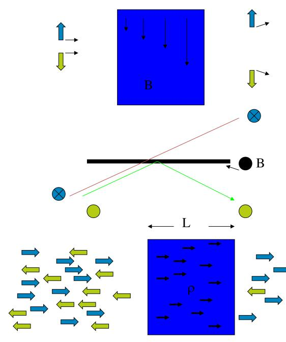
B gradients (Stern-Gerlach, sextupole magnets) electromagnetic  $F=(\mu \bullet \nabla)B$
