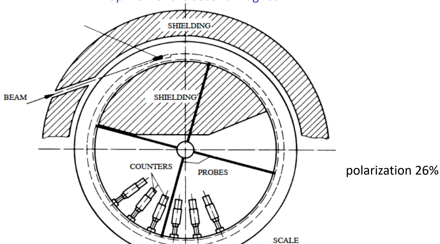
Fig. 17. The first muon storage ring: diameter 5 m, muon momentum 1.3 GeV/c, time dilation factor 12. The injected pulse of 10.5 GeV protons produces pions at the target, which decay in flight to give muons.
