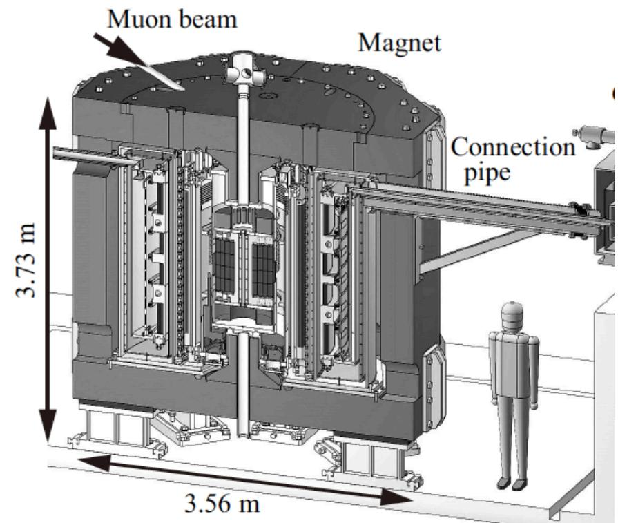
Fig. 8 Overview of the muon storage magnet
