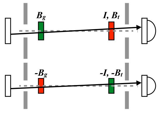
If  $d_{\theta}$ =0 and the apparatus is rotated, with  $\hat{I}$  and  $\hat{B}$  being reversed, then the transmission of neutrons in both states are equal.
