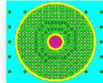
Three core models are considered in which selected Plutonium and minor actinide (Pu, Am, and Cm) loaded inside the inner zone
