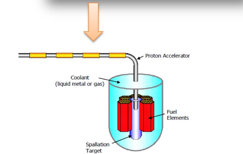
Schematic picture of an accelerator-driven system (ADS) concept
