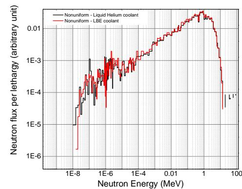
**Fig. 4c:** Neutron spectrum for the Nonuniform model with two coolant type (Liquid helium and LBE) in inner zone
