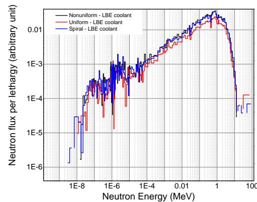
**Fig. 4b:** Neutron spectrum for the three models in inner zone in case of LBE coolant
