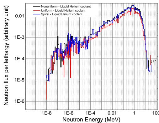
**Fig. 4a:** Neutron spectrum for the three models in inner zone in case of Liquid helium coolant
