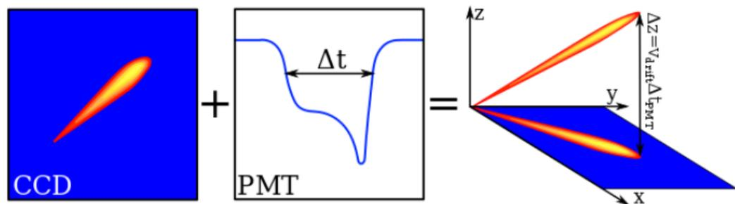
Reconstruction of the 3D tracks in the OTPC detector:
