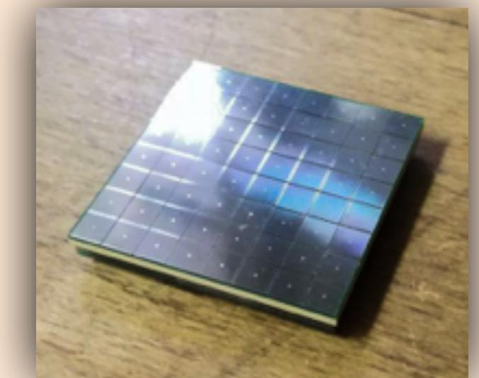
BGO -  $(\text{Bi}_4\text{Ge}_3\text{O}_{12})$
