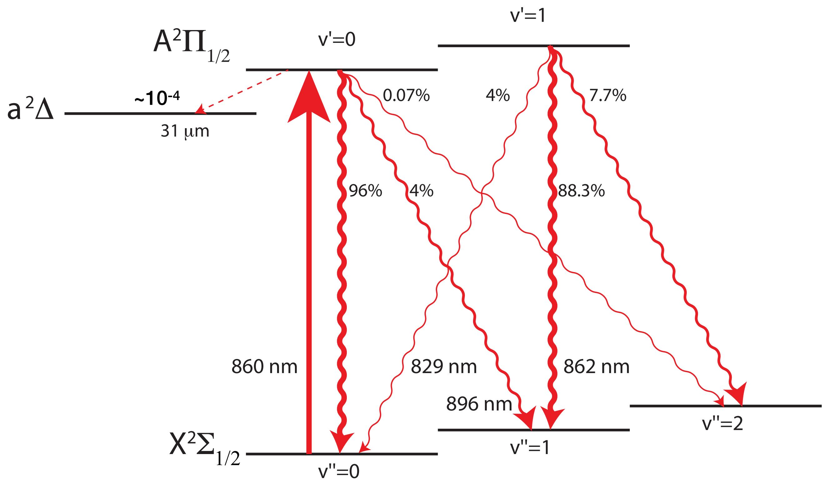
FC-factors sufficient for rapid (2 ms, 2000 photons) transverse laser cooling
