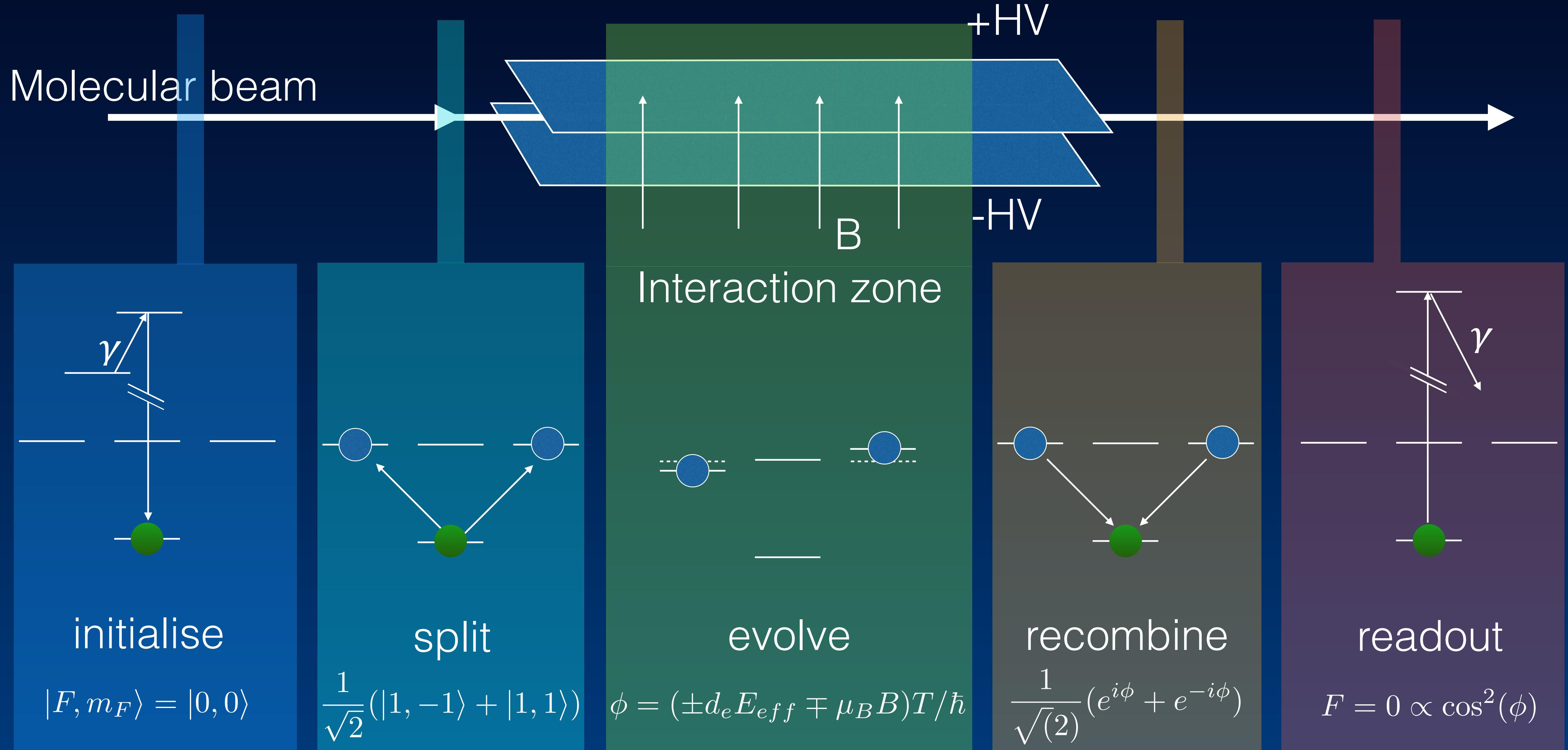
Interferometer phase  $\phi = (\pm d_e E_{eff} \mp \mu_B B)T/\hbar$
