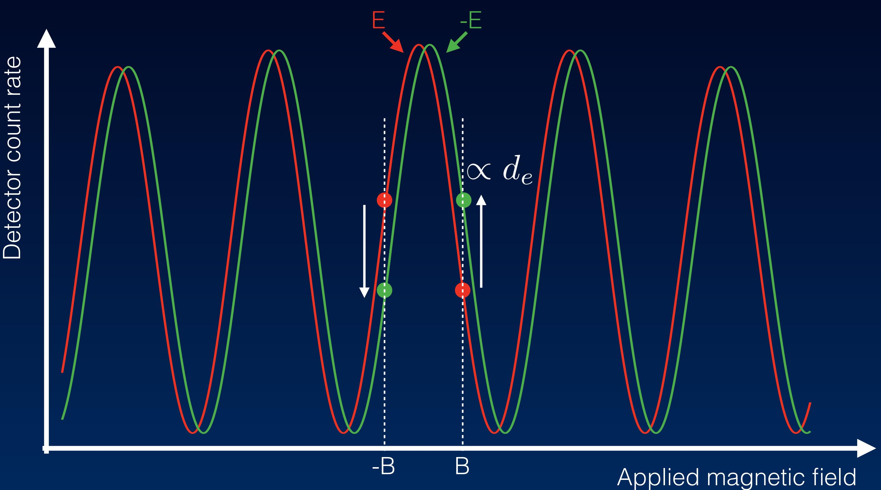
$$\text{Interferometer phase } \phi = (\pm d_e E_{eff} \mp \mu_B B)T/\hbar$$
