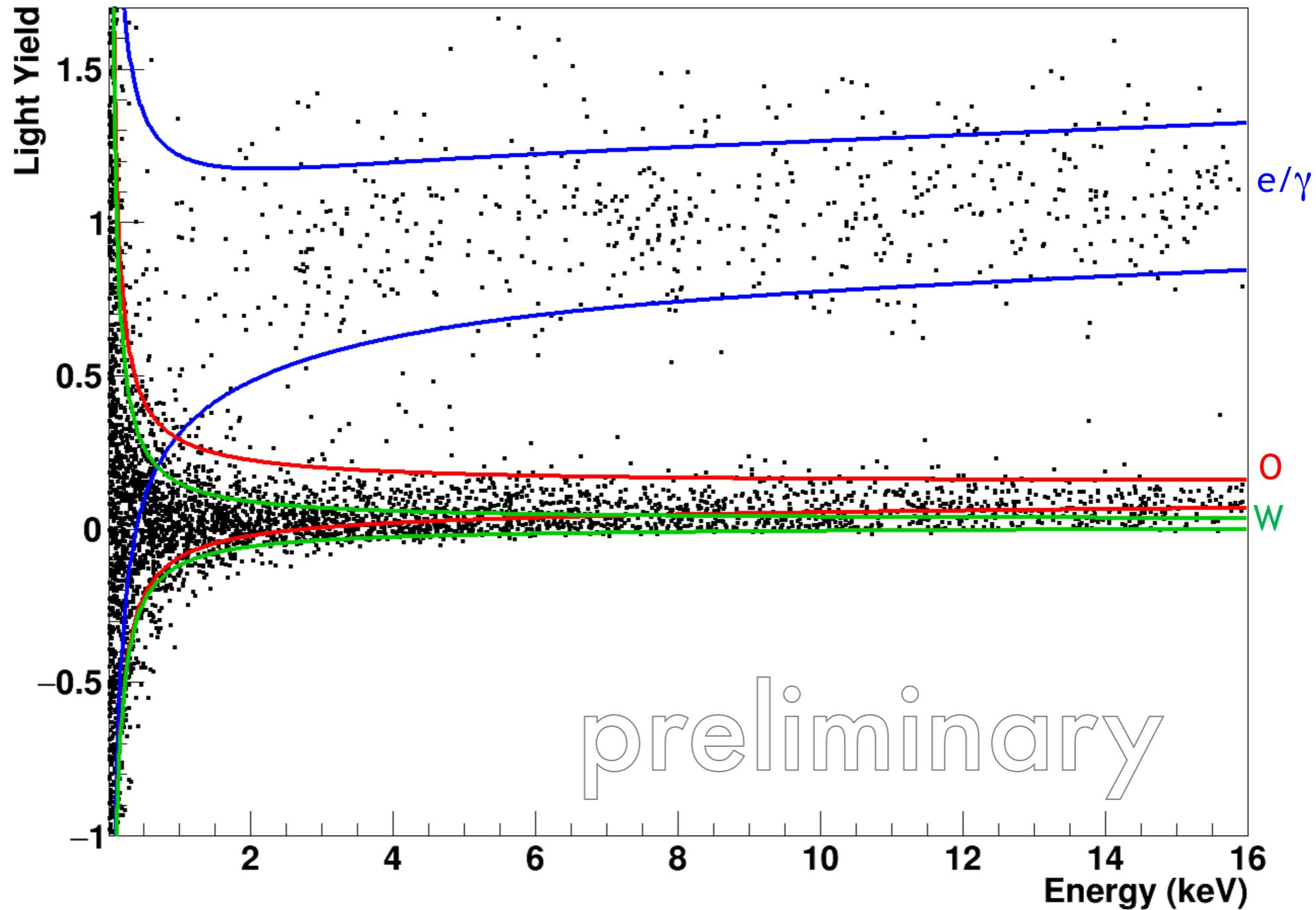
Quenching factors measured with neutron beam
