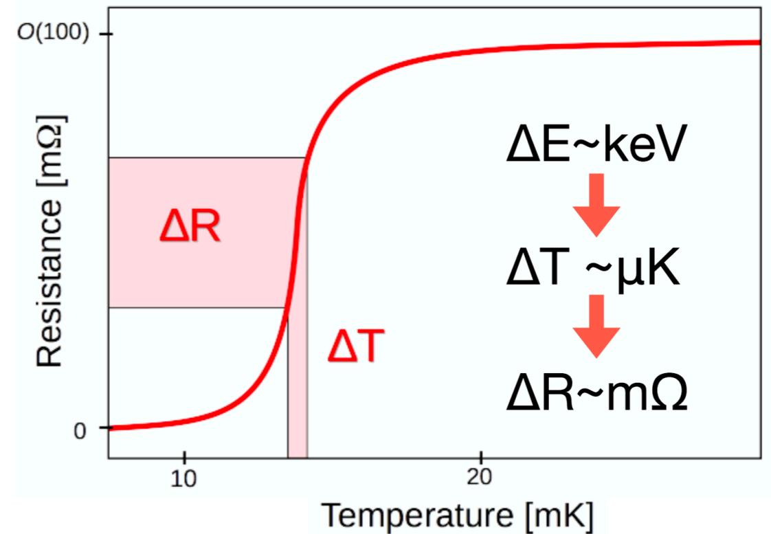
Detection of temperature rise with **TES** (Transition Edge Sensor) sensors operated at the phase transition from normal to superconducting.
