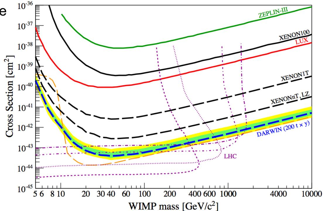
Upper limits on the spin-dependent WIMP-neutron cross section of ZEPLIN-III, XENON100 and LUX as well as projections for XENON1T, XENONnT, LZ and DARWIN. For the 14 TeV LHC limits for the coupling constants  $g_\chi = g_i = 0.25, 0.5, 1.0, 1.45$  (bottom to top) are shown.
