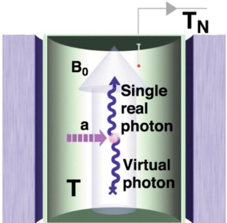
$$P_{\text{out}} \sim g^2 |B_0|^2 \rho_{\text{DM}} V Q / m_a$$
