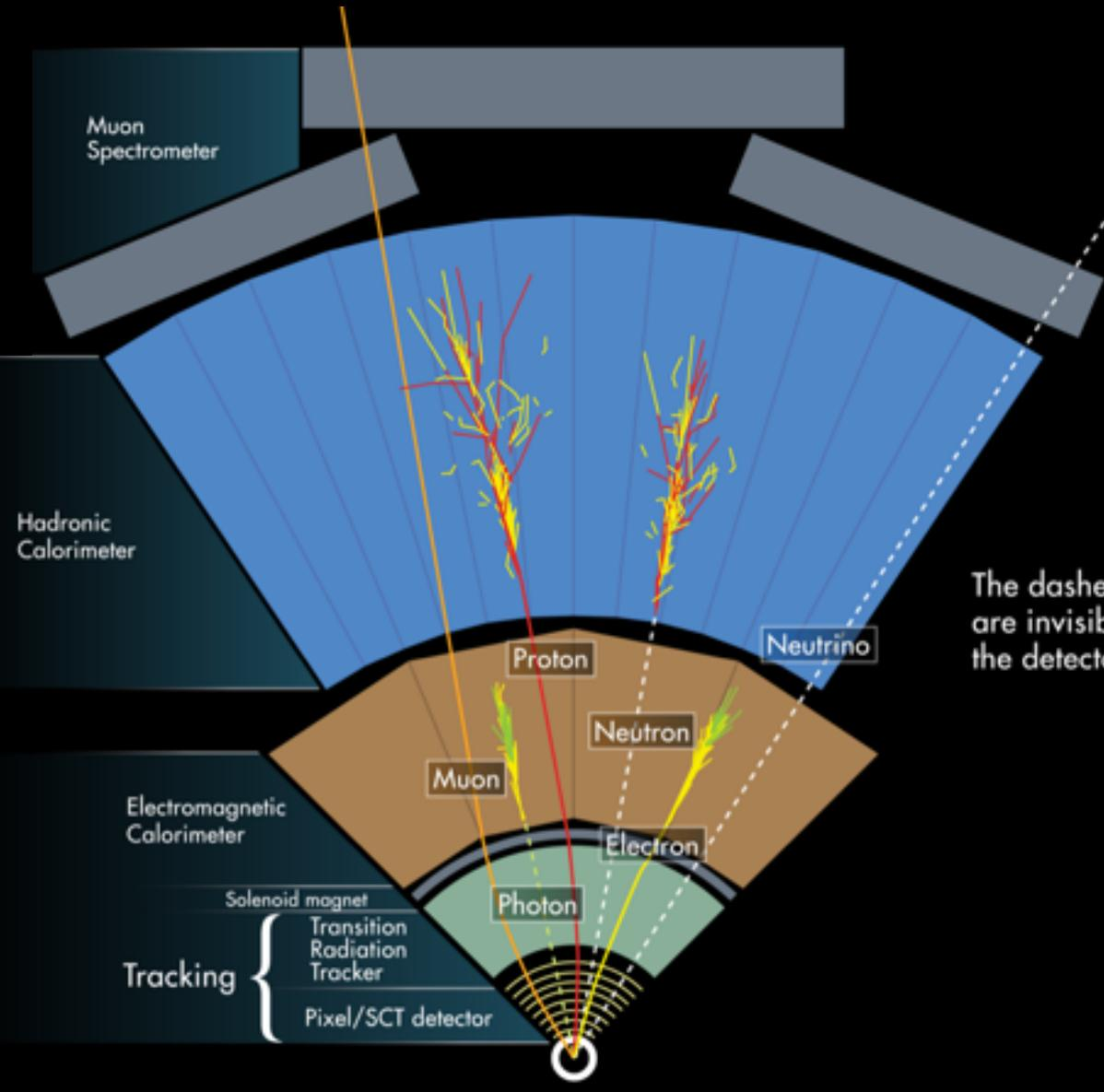
**Muon-Detectors:** Identification and precise momentum measurement of muons outside of the magnet
