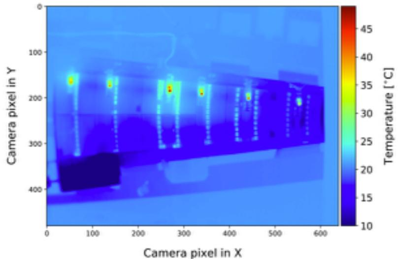
IR picture of thermo-mechanical prototype
