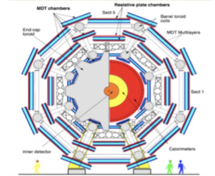
Fast detector systems detect possible interesting signature and trigger the inner detector systems to be read out. Other events are discarded.
