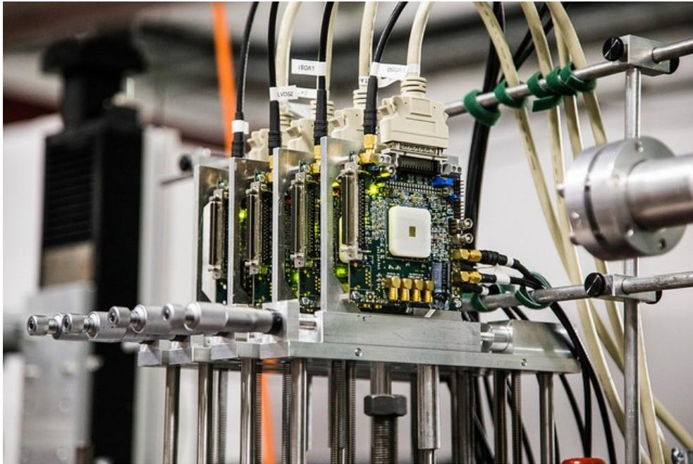
4-layer HV-MAPS pixel detector (3x3 mm)
