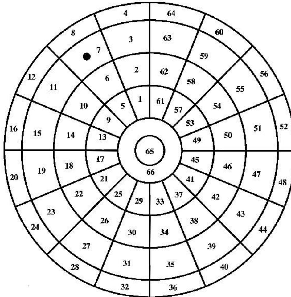
. 66 pads in total. The central pad is 20 mm in diameter
