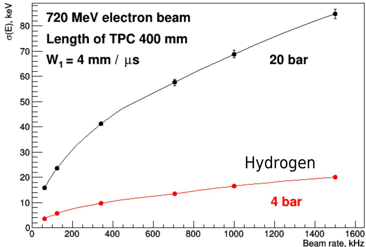
Expected TPC energy resolution in the main experiment at 2 MHz beam rate
