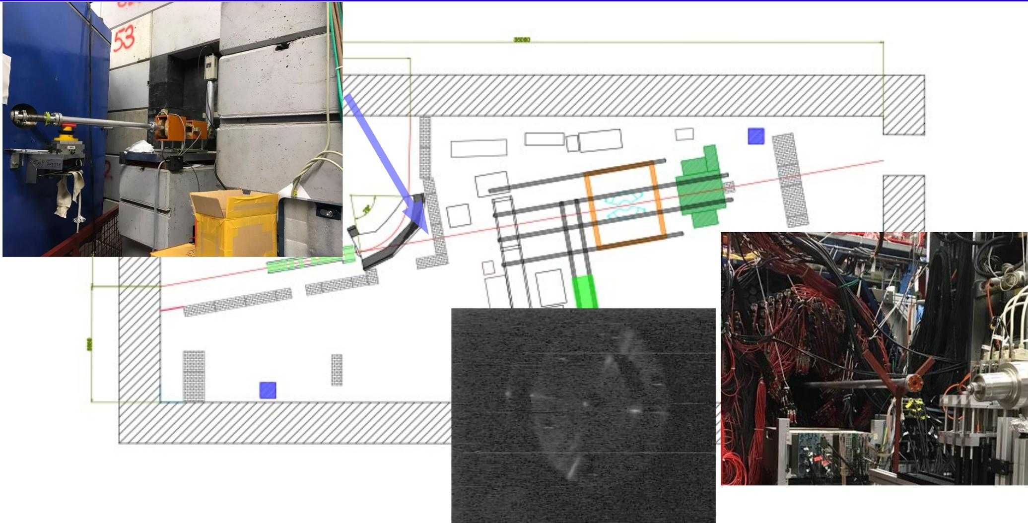
→ One horizontal and one vertical steering magnets before tagger wall, luminescent screens for steering, ionization chamber connected to the interlock (M. Dehn)
