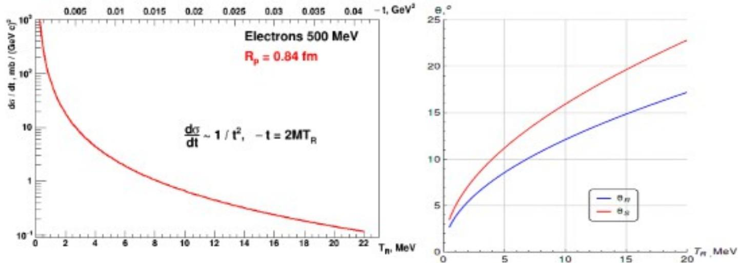
Figure 2: Left panel: differential cross section of the  $ep$  elastic scattering calculated for  $\varepsilon = 500$  MeV with electric and magnetic form factors represented by expansion Eq. 2. Right panel: Scattering electron and recoil proton angles as function of the recoil proton energy.
