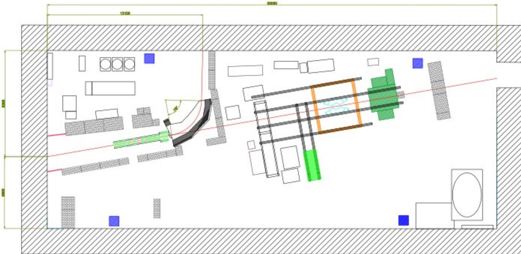
Replaced the photon beamline in the A2 Hall with a temporary electron beamline
